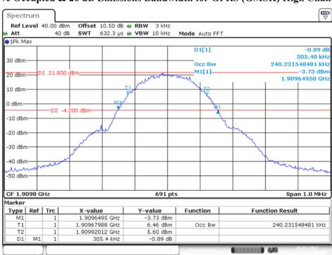
99% Occupied & 26 dB Emissions Bandwidth for GPRS (GMSK) High Channel
