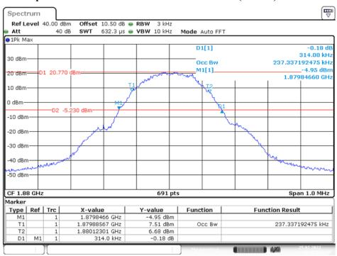
99% Occupied & 26 dB Emissions Bandwidth for GSM (GMSK) Middle channel
