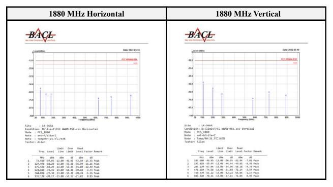
EUT emissions correction = Read Level Level = Read Level + Factor (Antenna Factor + Cable Loss – Amplifier Gain.)
