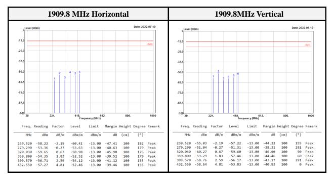
EUT emissions correction = Reading
