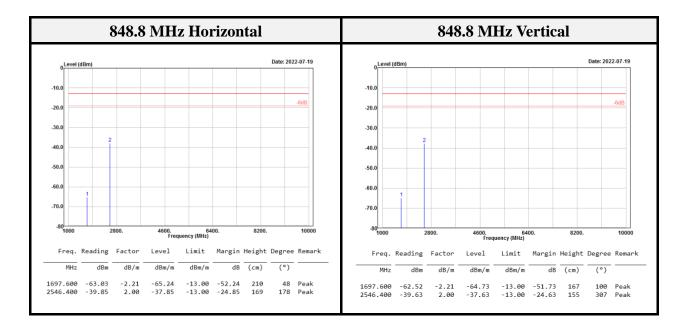
EUT emissions correction = Reading Level = Level + Factor (Antenna Factor + Cable Loss – Amplifier Gain.)
