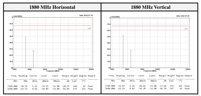
EUT emissions correction = Reading Level = Level + Factor (Antenna Factor + Cable Loss – Amplifier Gain.) Margin = Level – Limit.
