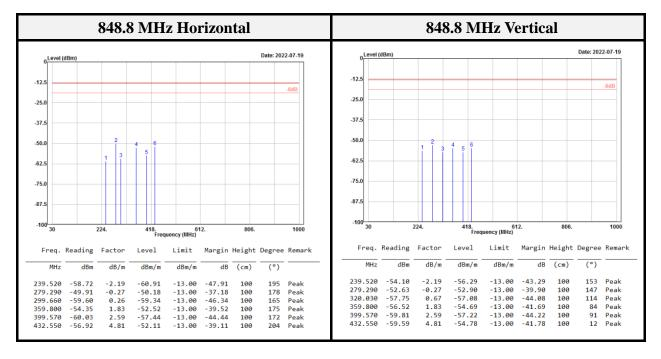
EUT emissions correction = Reading
