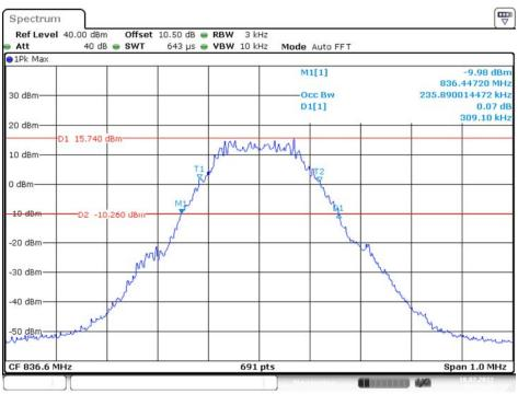
99% Occupied & 26 dB Emissions Bandwidth for GPRS Middle channel
