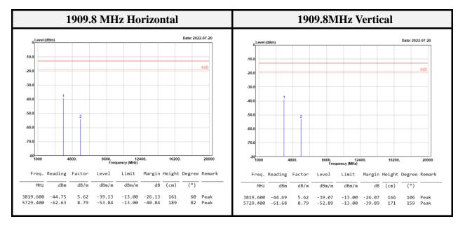
EUT emissions correction = Reading Level = Level + Factor (Antenna Factor + Cable Loss – Amplifier Gain.)
