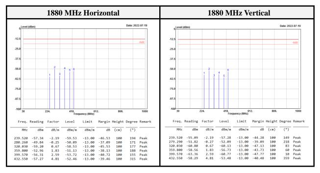
EUT emissions correction = Reading Level = Level + Factor (Antenna Factor + Cable Loss – Amplifier Gain.) Margin = Level – Limit.
