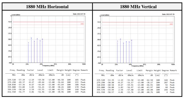
EUT emissions correction = Reading Level = Level + Factor (Antenna Factor + Cable Loss – Amplifier Gain.) Margin = Level – Limit.
