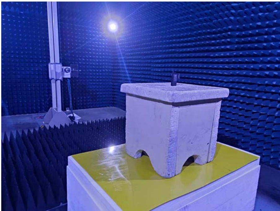
Photo of Radiated Emission Measurement Above 1GHz
