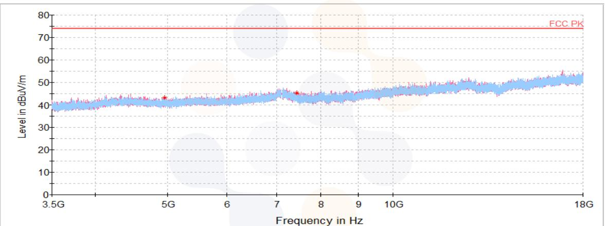
**Test results (Above 1 000 MHz)\_2 MBits/s(37 Bytes)****2 402 MHz**
