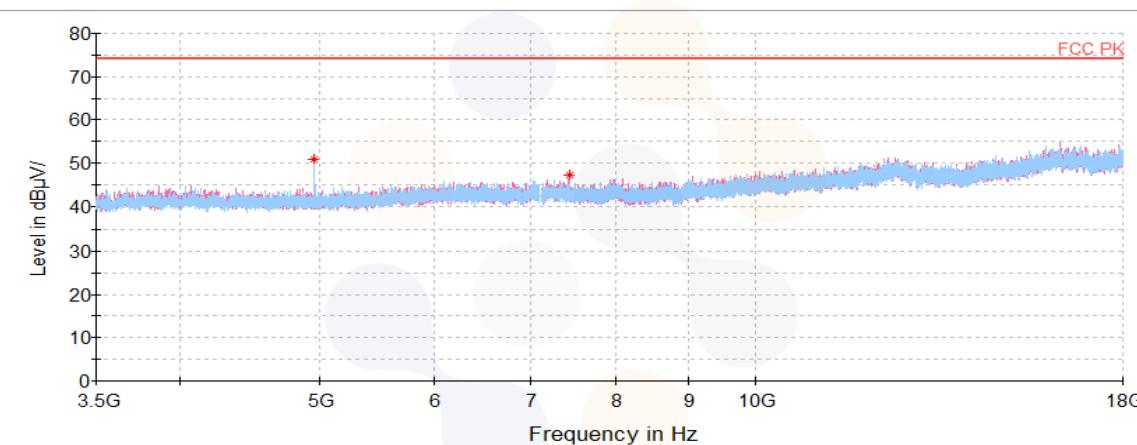
**Test results (Above 18 GHz) – Worst case: 1 MBits/s(37 Bytes) 2 480 MHz****Horizontal/Vertical for 18 GHz ~ 26.5 GHz**
