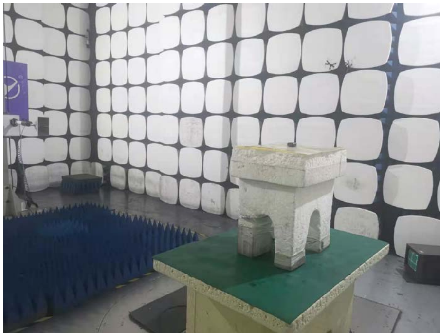
Spurious Emission Test Setup (Above 1GHz)
