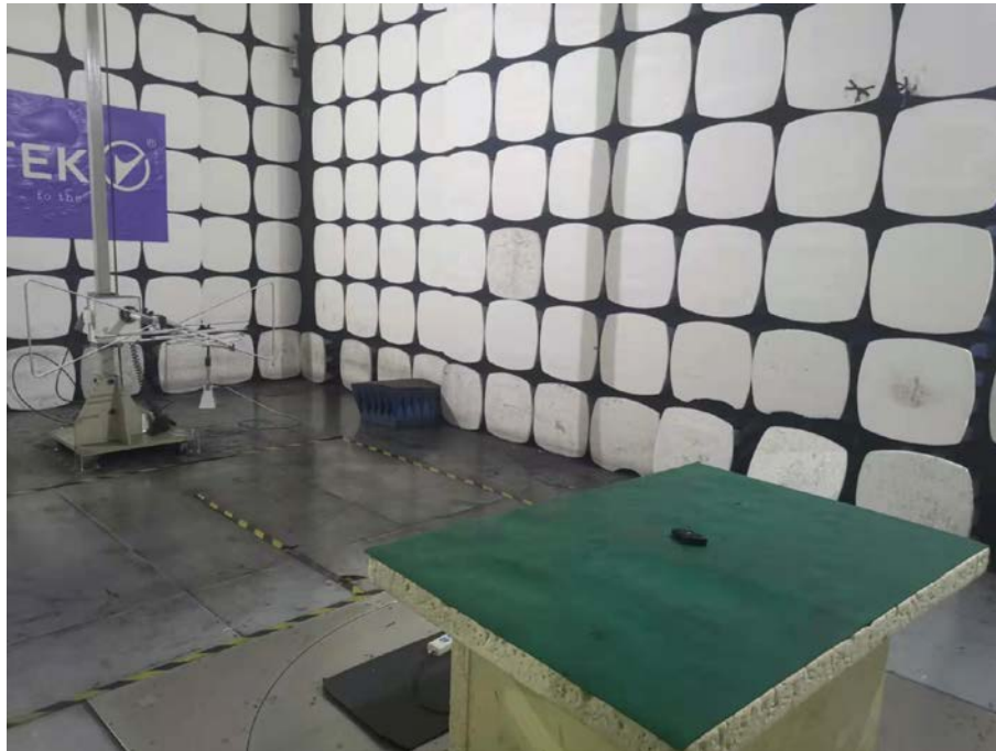
Spurious Emission Test Setup (Below 1GHz)
