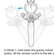
button, tilt the remote control to the left, and turn the aircraft's head to the left; The remote control tilts to the right, and the aircraft turns its head to the right
