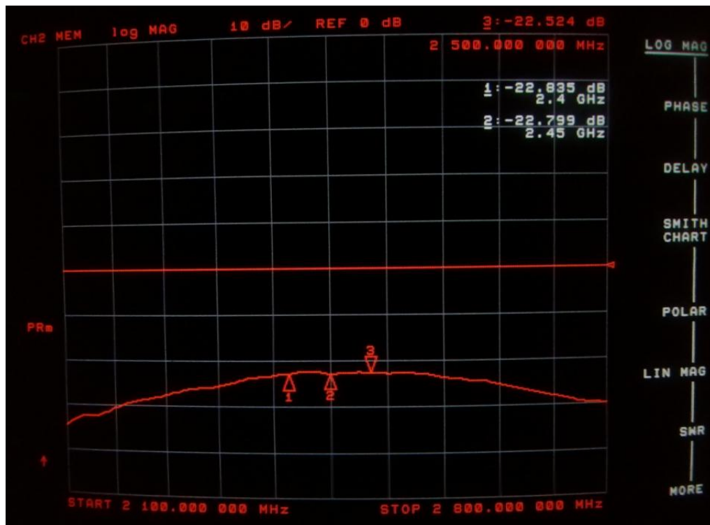
Isolation of WiFi-A and WiFi-B antenna (2.4G)
