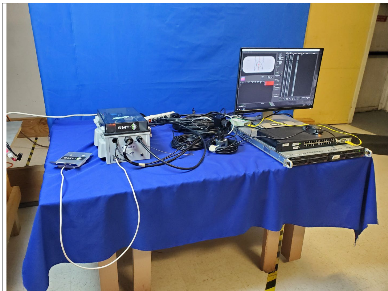
EUT setup with support units
