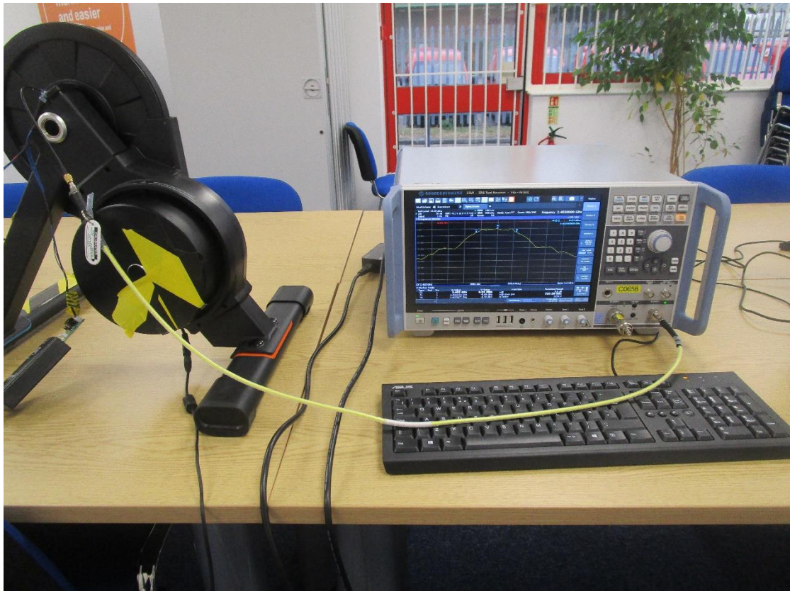
Arrangements for conducted tests – antenna port (Output power, conducted spurious, occupied bandwidth etc.)
