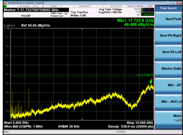
4-18 GHz, Vertical Antenna Vertical EUT, Channel 19
