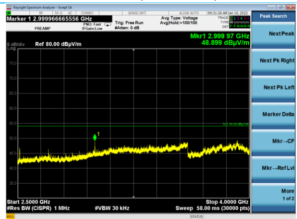
2.5-4 GHz, Vertical Antenna Vertical EUT, Channel 19
