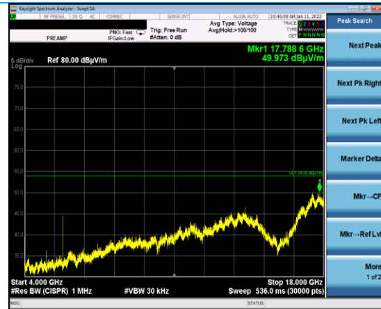
4-18 GHz, Vertical Antenna Vertical EUT, Channel 39
