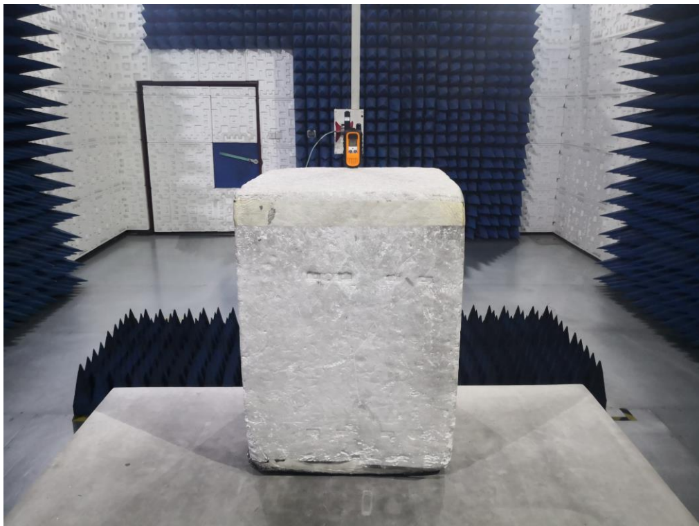
RADIATED EMISSION TEST SETUP ABOVE 1GHz
