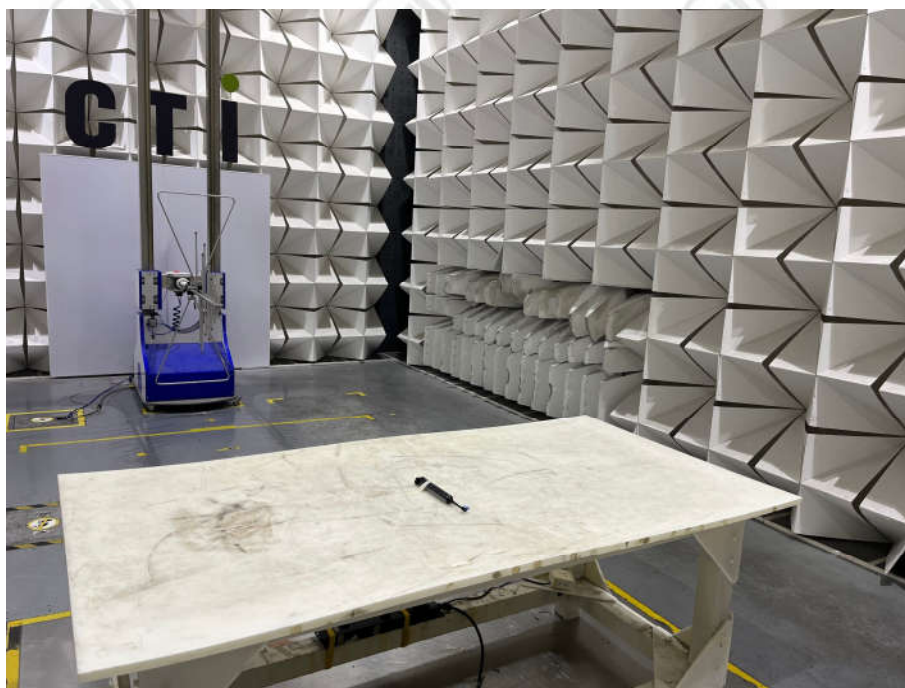
Radiated spurious emission Test Setup-1(Below 1GHz)
