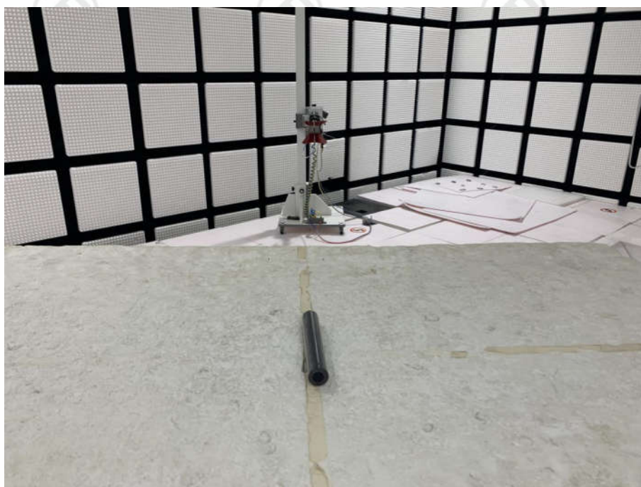
Radiated spurious emission Test Setup-2(Above 1GHz)
