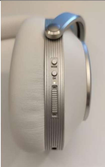
Right Ear-Cup Rear: Mode Button Digital Assistant Activation Button Bluetooth Switch and Indicator
