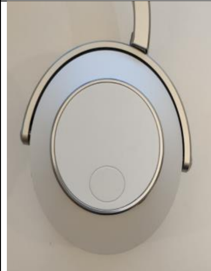
Right Ear-Cup Side: Large Touch Area: Play / Pause, Call Control, Volume Up/ Down, Next / Previous Title Small Touch Area: Transparent Mode ON / OFF
