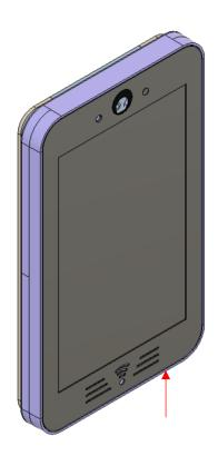
Put the security screw back (from Step 1) to secure the display after mounting.
