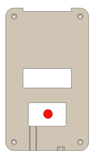
Make a hole for the cable in the lower square on the back plate like shown in the picture above.
