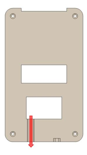
If installation is done without having the cable coming in from behind the display, place the cable inside the groove of the backplate as shown in the picture above.
