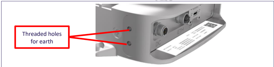
Figure 5. Earthing points: TN001xC In-train unit
