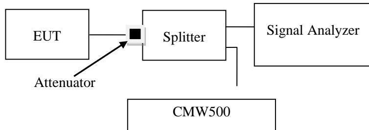
Note: the worst path loss (Attenuator, cable loss and splitter inset loss) among the test frequency range was added into plots.
