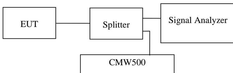
Note: the worst path loss (cable loss and splitter inset loss) among the test frequency range was added into plots.
