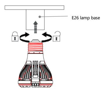
Put the lamp holder screwed to the E26 lamp base.
