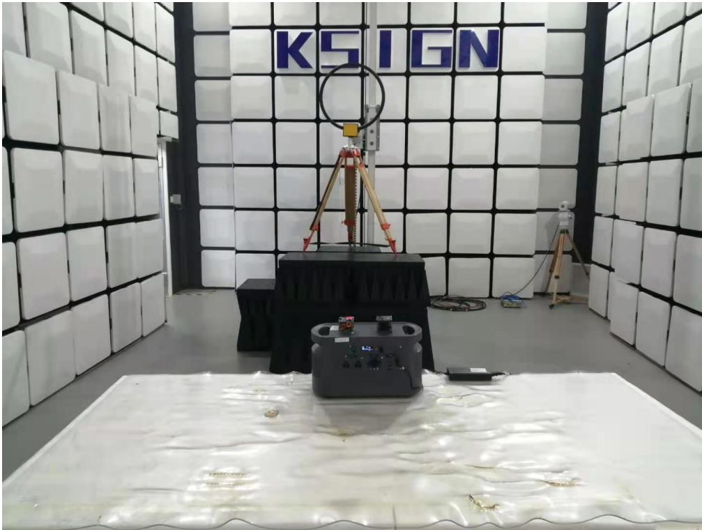
Radiated Measurement (Below 30MHz)
