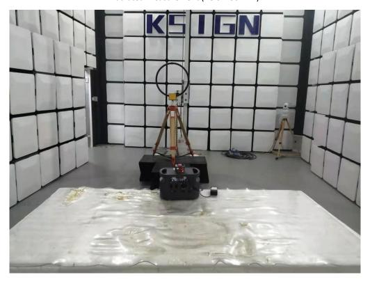
Radiated Measurement (Above 30MHz)
