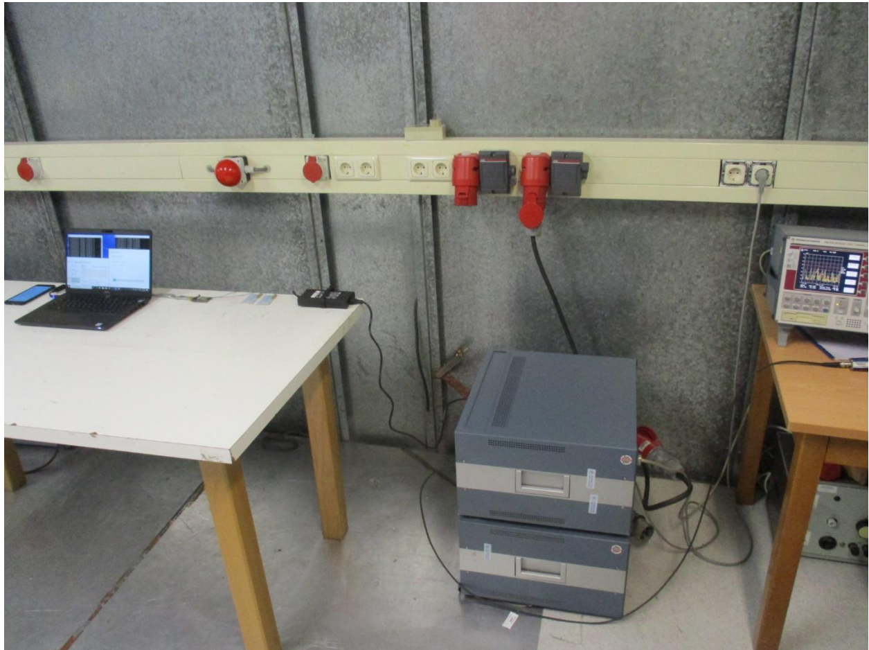
Photo 5: Photograph conducted emissions 0.15-30 MHz
