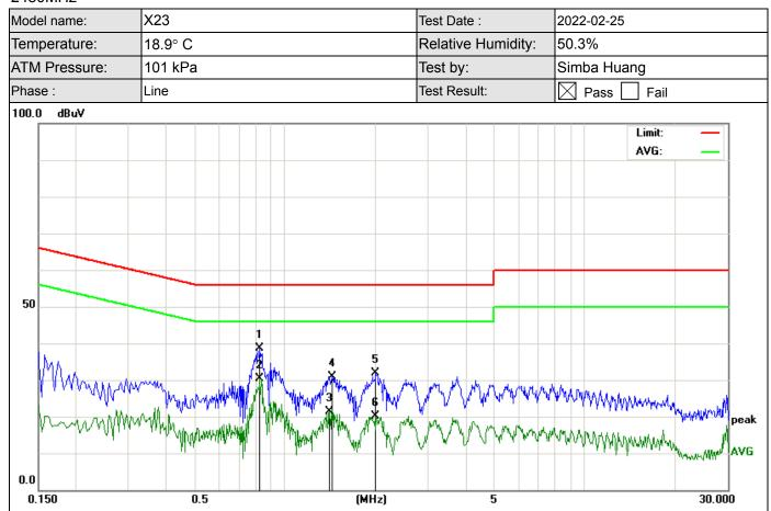
Remark: Factor = Antenna Factor + Cable Loss - Pre-amplifier.
