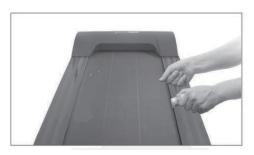
is better to maintain like this every 30 hours working of the machine. This can save lifetime of parts properly.
