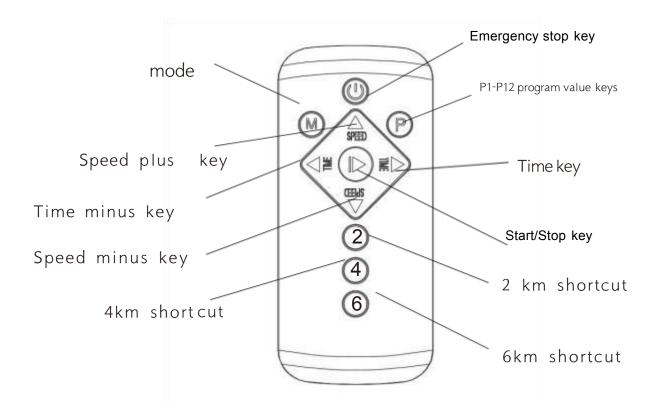
Emergency Stop Key: Press this key in the event of an emergency or when an emergency shutdown is required
