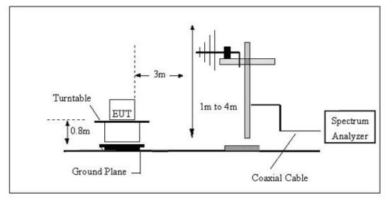
(C) Radiated Emission Test-Up Frequency Above 1GHz
