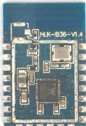
Figure 1: Position and effect of HLK-B36 onboard antenna
