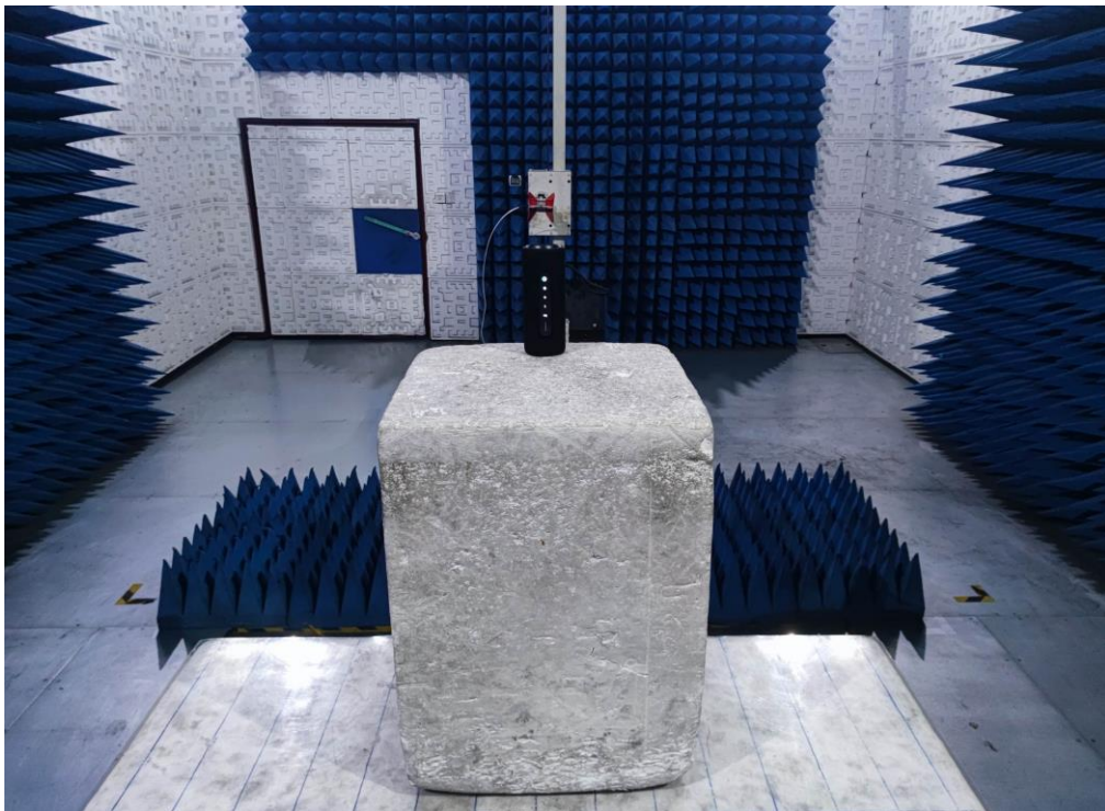
RADIATED EMISSION TEST SETUP ABOVE 1GHz
