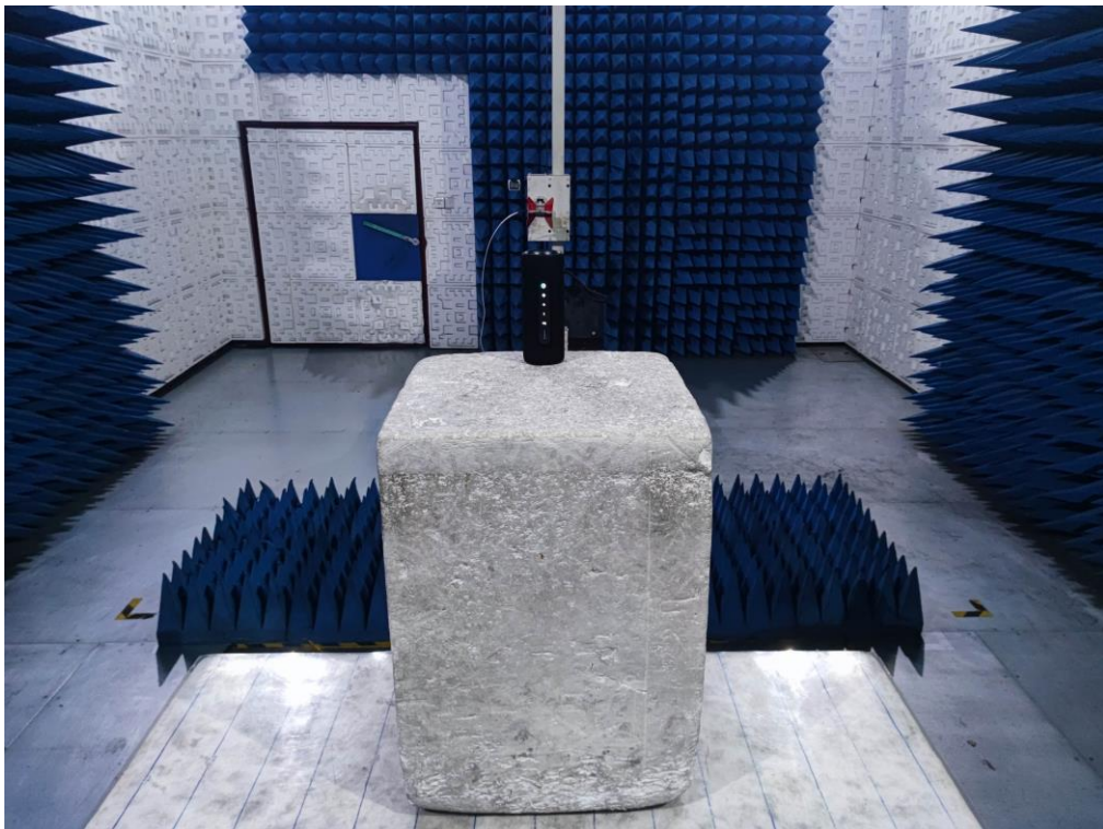
RADIATED EMISSION TEST SETUP ABOVE 1GHz
