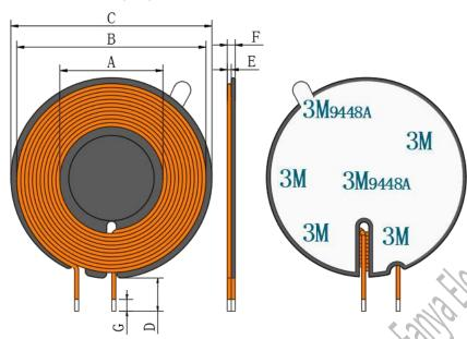
A  $21.46\pm0.5$ B  $39.3\pm0.5$ C  $42.4\pm0.4$ D  $55\pm1.5$ E  $0.8\pm0.2$ F 2.2Max (No separation paper thickness)
