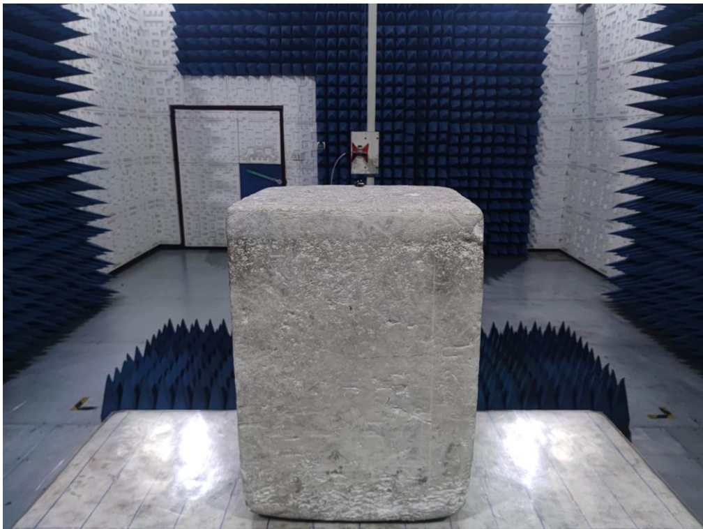
RADIATED EMISSION TEST SETUP ABOVE 1GHz
