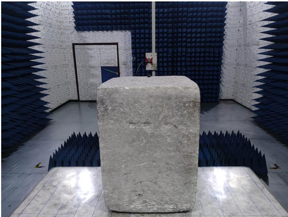
RADIATED EMISSION TEST SETUP ABOVE 1GHz
