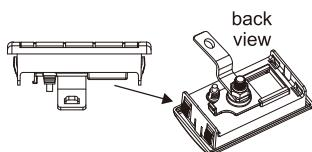
2. Slide the Bluetooth® controller into the hook
