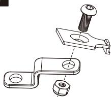
1. Install "Z" shaped bracket threaded on to the Bluetooth® controller hook. (packed with Bluetooth® controller.)
