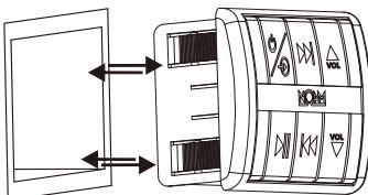
**STEP1** Decide the place for Bluetooth® remote installation. Draw and cut the size into 85 x 49mm (L x W)
