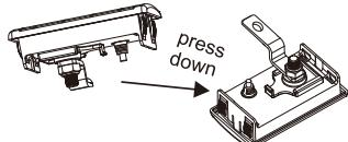
3. Press down the Bluetooth® controller hook and then slide out the Bluetooth® controller box at the same time to remove the Bluetooth® controller
