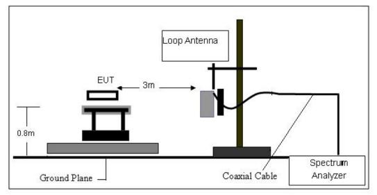
(B) Radiated Emission Test-Up Frequency 30MHz~1GHz
