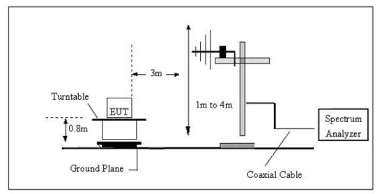
(C) Radiated Emission Test-Up Frequency Above 1GHz
