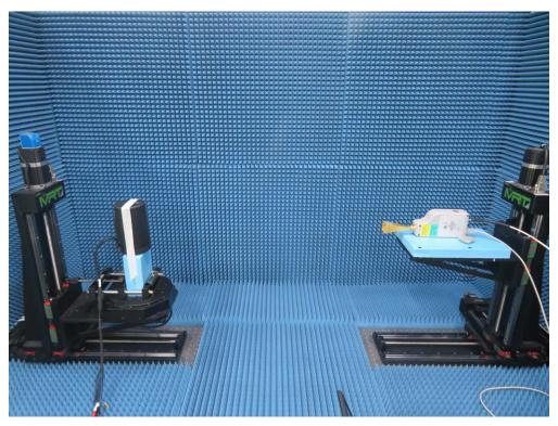
Description: Radiated Spurious Emission Test Setup for Between 75GHz ~ 100GHz
