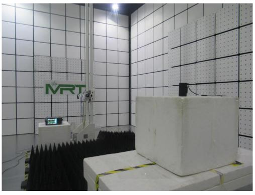
Description: Radiated Spurious Emission Test Setup for Between 40GHz ~ 50GHz
