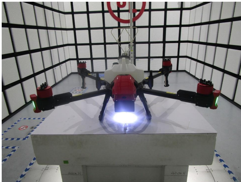
RADIATED RF MEASUREMENT SETUP (Below 1 GHz)
