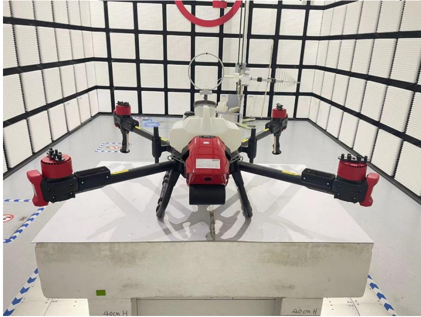
RADIATED RF MEASUREMENT SETUP (Below 1 GHz)
