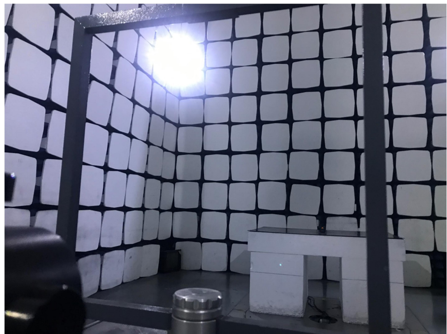
Radiation Emission Test Setup (Below 30MHz)
