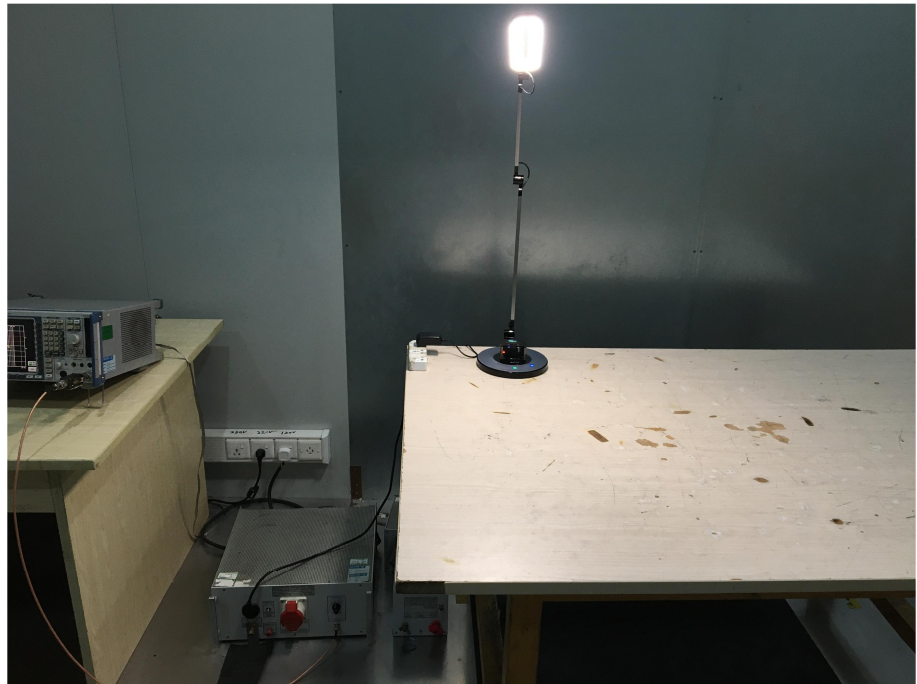
Conducted Emission Test Setup
