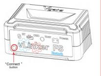
Step 2: Open the Bluetooth settings. Search for the device name "vLinker FS 23199" and click Pair. (23199 is the product serial number, each product has a different serial number)
