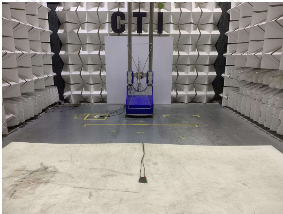
Radiated spurious emission Test Setup-1(Below 1GHz)
