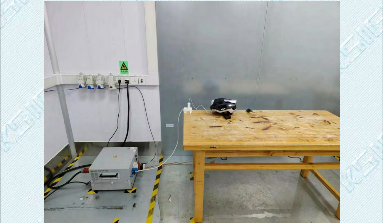
Conducted Emission at AC power line
