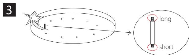
long side connects to the holder, and short side connects to the segments, wire gets through this vibe.
