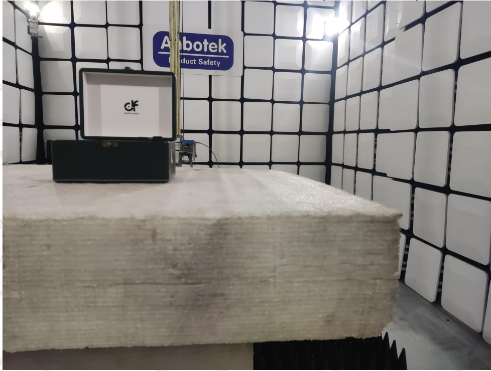
Photo of Radiation Emission Test (above 1GHz)
