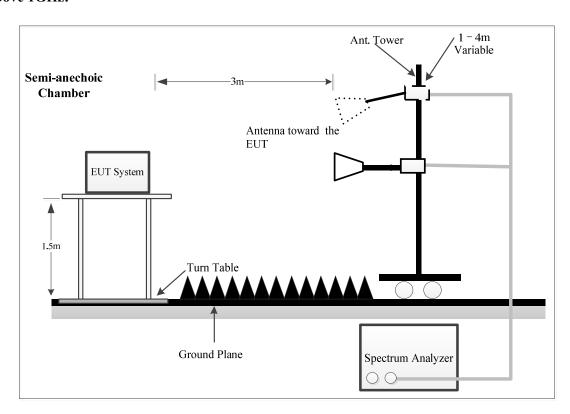
The radiated emissions were performed in the 3 meters distance, using the setup accordance with the ANSI C63.10-2013. The specification used was the FCC 15.209, and FCC 15.247 limits.
