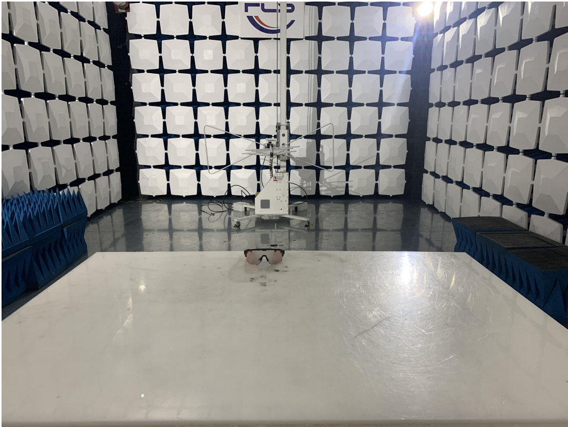
Above 1GHz for radiated emission test setup
