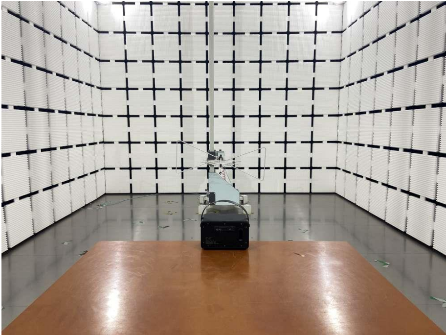
Radiated Emission Test View Below 1GHz
