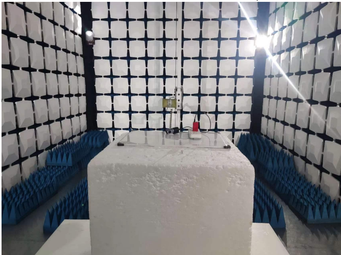
Above 1GHz for radiated emission test setup
