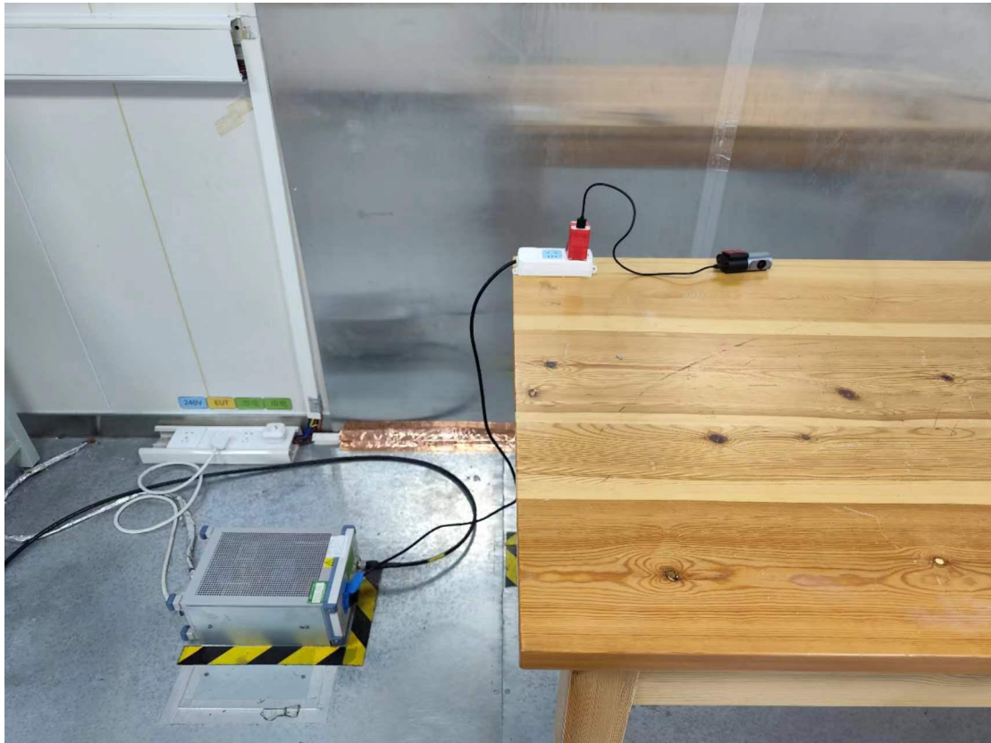
Conducted emission test setup
