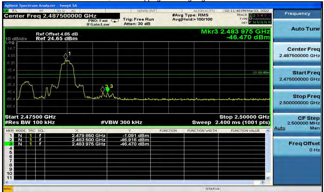
\pi/4 -DQPSK No-hopping Band edge-right side
