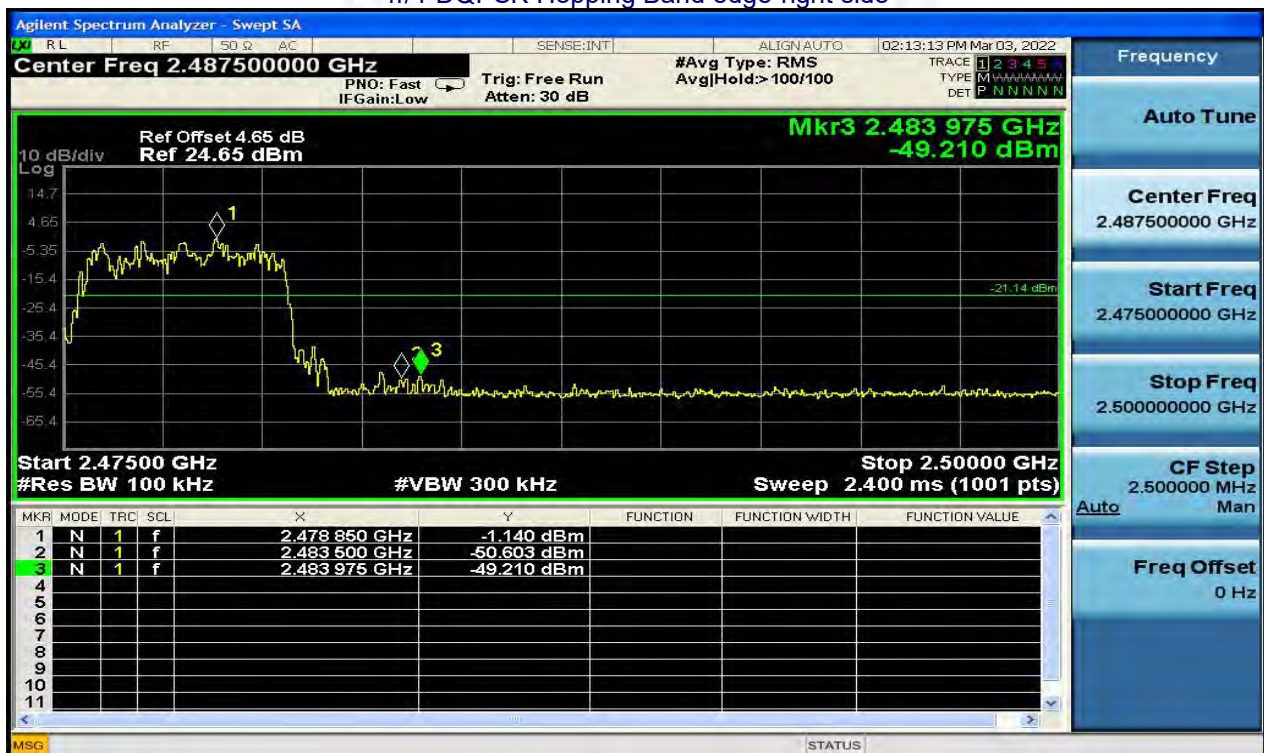
\pi/4 -DQPSK Hopping Band edge-right side
