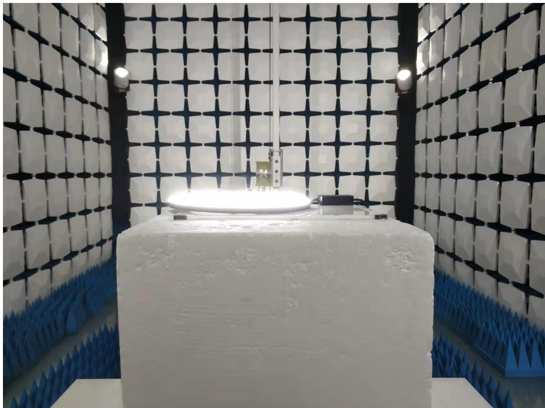
Above 1GHz for radiated emission test setup
