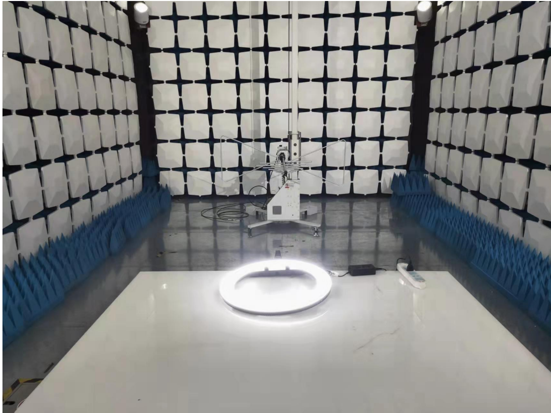
Below 1GHz for radiated emission test setup
